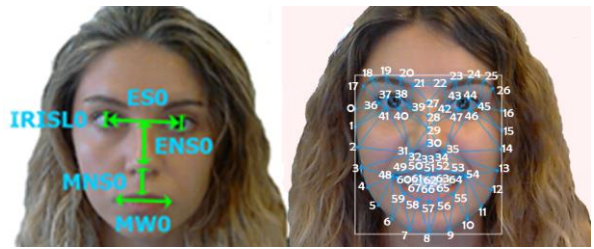
Fig. 3. FAPUs (left) and landmarks (right) provided by the BRFv4.
